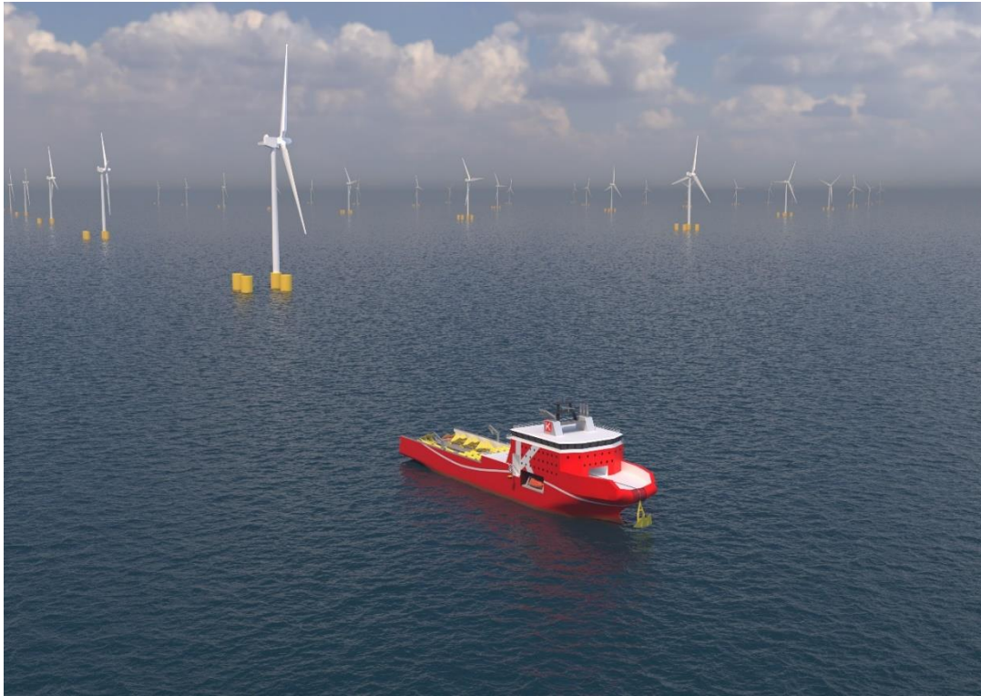
Image of the multi-functional floating offshore windfarm support vessel (MFSV) *3 , expected to be used in mooring installation
